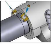
quality of the probes. If the shaft is inspected and found to be clean and smooth then this location may be used for measurement. The advantages of this mounting style are the low cost and the easy access to the probes.
